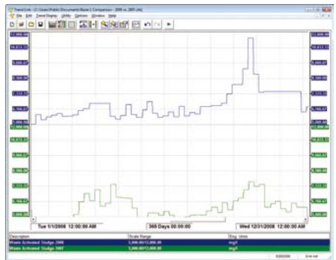
Figure 3: Being able to compare data from a previous run (2008 v 2007) allows an engineer to spot what was different.
